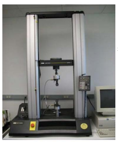
**Instron Universal Tester** QA equipment is used to determine the break strength of paper products, linens (towels, washcloths, sheets, pillowcases) and plastic can liners; tear strength of linens; % elongation (stretch) of can liners before they break/tear.
